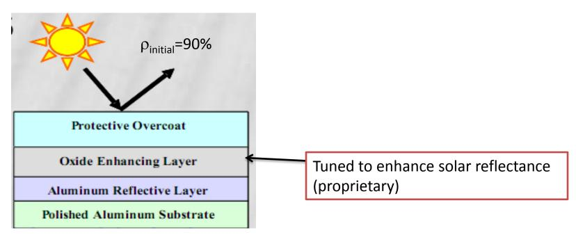
**Drawbacks:** more durability testing needed, low  $\rho_{initial}$
