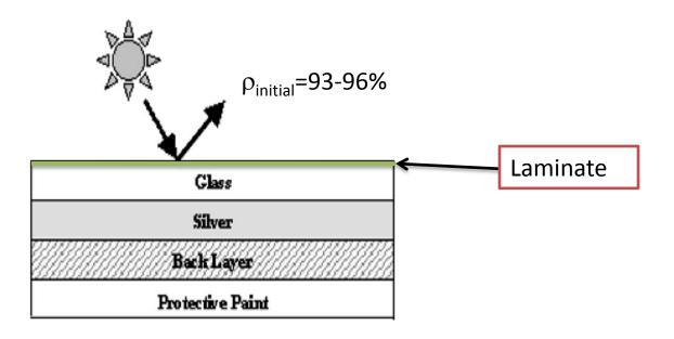
**Drawbacks:** fragile and difficult to handle, corrosion after 2 years where no adhesive, adhesive effects  $\rho$  over time
