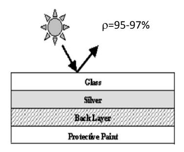
**Drawbacks:** heavy, cost could be reduced, and silver's absorption band
